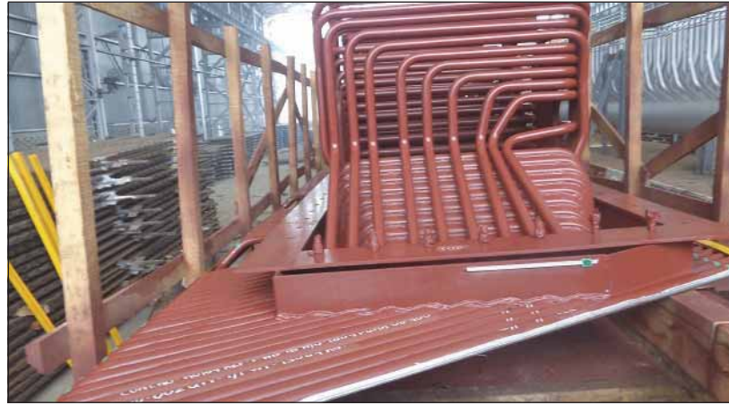
Manufacturing of Super Critical Boiler at Alstom India Ltd., Durgapur
